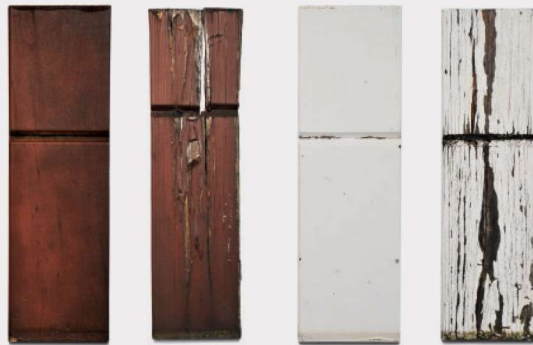
Acetylated wood Unmodified wood Acetylated wood Unmodified wood Translucent WB Acrylic Coating Opaque WB Acrylic Coating
