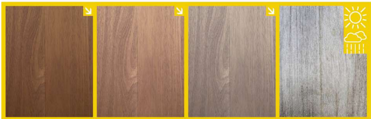
Excellence - After Installation | Unoiled wood exposed to UV light
